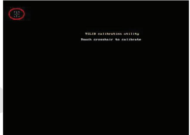
※ During the correction, please do perform the operation according to the positions of crosses. Otherwise, the touching panel will be unable to work normally after the correction.
